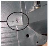
6. To install the front and rear doors, first install the door bearings into the bottom of the door frames. Install the door onto the bearing and then pull down the spring loaded door bearing to install the top of the door.
